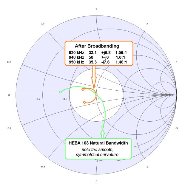
The Smith Chart above shows the actual measured bandwidth of the HEBA103, within the 20 kHz channel of WQVR, in green. Kurt Gorman of Phasetek, WWAS Chief Engineer, recently redesigned the WQVR Antenna Tuning Unit with bandwidth-flattening design technology, so that All-Digital AM transmission performance will be quite good, as shown in orange.
